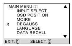
**INPUT SELECT** toggles between D-Sub and BNC video sources, giving you the option of switching between two monitors (see page 6). Press [▼] or [▲] to select one of these options.
